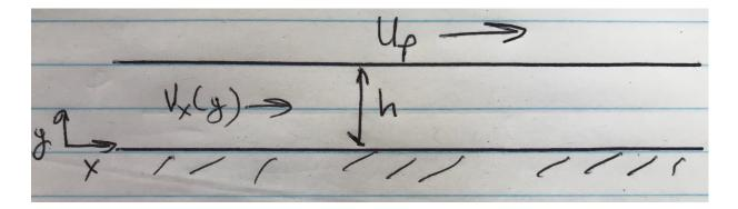
b. If the viscosity of the liquid is 0.003 kg/(m-s), h = 0.1 mm and  $U_p = 3$  cm/s, what is the shear stress in the channel?
