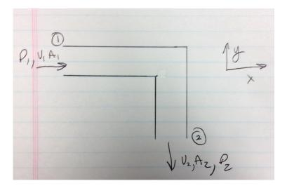
Consider first that area does not change around the bend and that the flow does not have any viscous losses.
