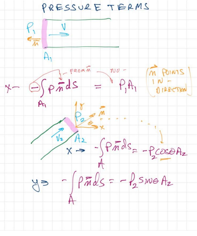
Fxî+Fxi ((n. ~)ds = COMBINATION OF PRESSURE AND SHEAR STRESS VSUALLY CAN'T EVALUATE INTEGRALS EXACTLY SO: COMPLETE BALANCE -9 1,2A, +8 1/2 COS OA2 = P, A, - P2A2 COSO 0 + 8 V2 SINDAR2 = -P2 AZSING +FA A USUAL QUESTION IS "FIND F
