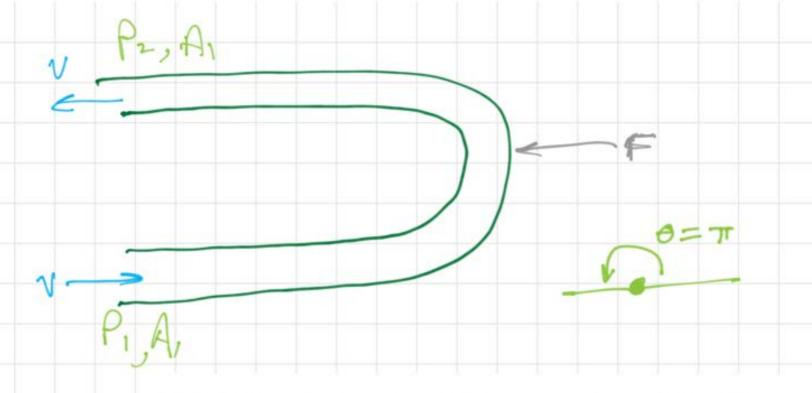
Momentum equations for single flow inlet in + x direction.
