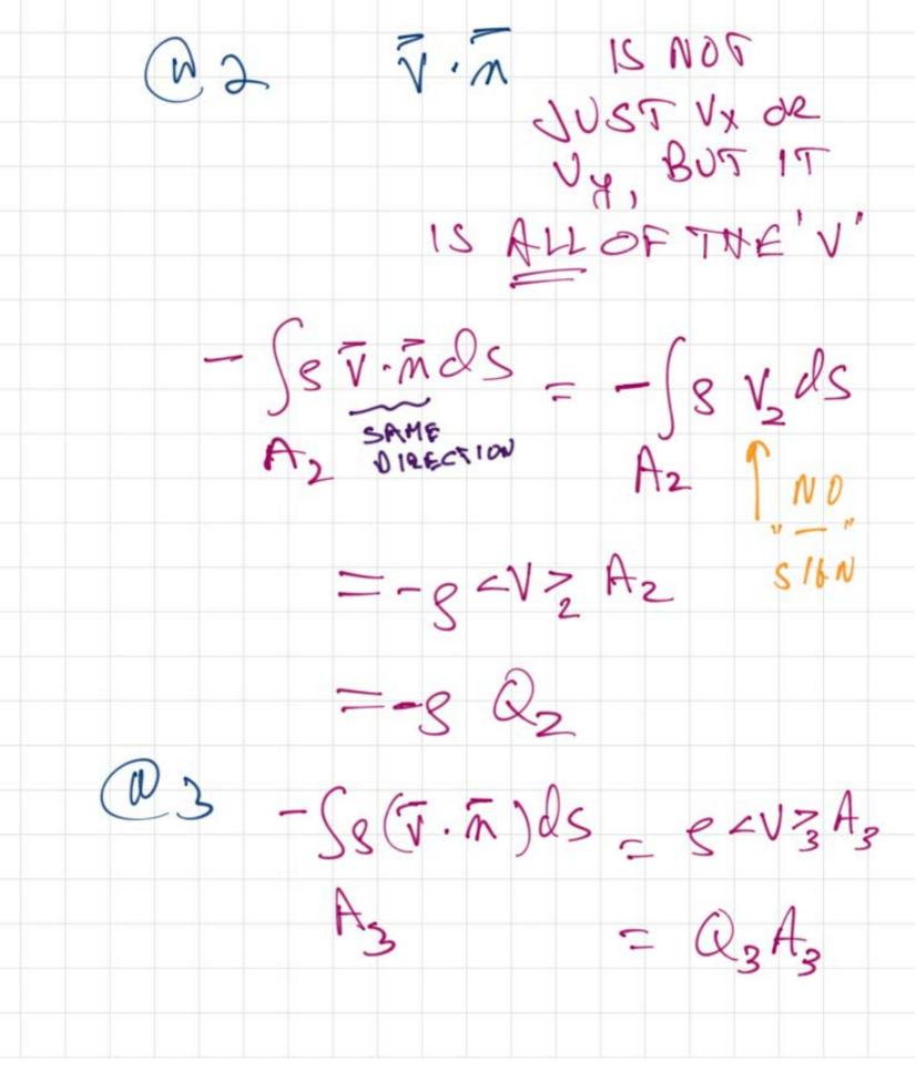
THE ANSWER MATCHES WHAT WEEXPECT 0= 8 < V > A, - 8 < V > A2 - 8 < V73 A3 2 m  $= S \leq 2 \sqrt{2} A_i - S \leq 2 \sqrt{2} A_j$ USEFUL IN THIS FORM, FOR TURBULENTFLOWS IN PIPES & DUCTS, VELOCITY PROFILE IS USUALLY "FLAJ" ENDUGH TO JUST WRITTE "V," AS A SINGLE VALUE.
