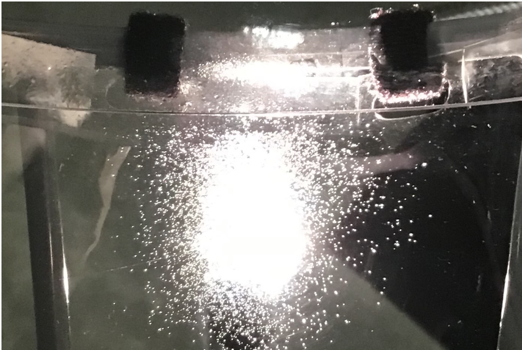
Figure 1. Spray pattern associated with maximum exhalation, pursed lips. A very large quantity of droplets are captured by both the mouth guard and the visor.
