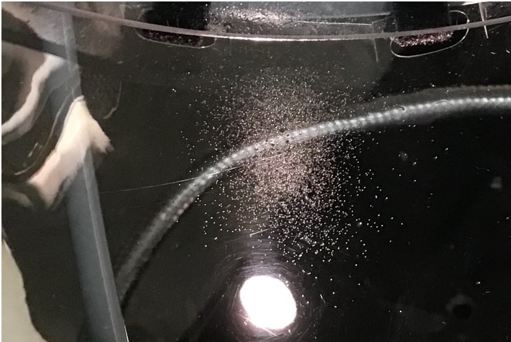
Figure 2. Spray pattern associated with clearing breath and pursed lips. The number of droplets is less than that for maximum exhalation, however the distribution is similar.
